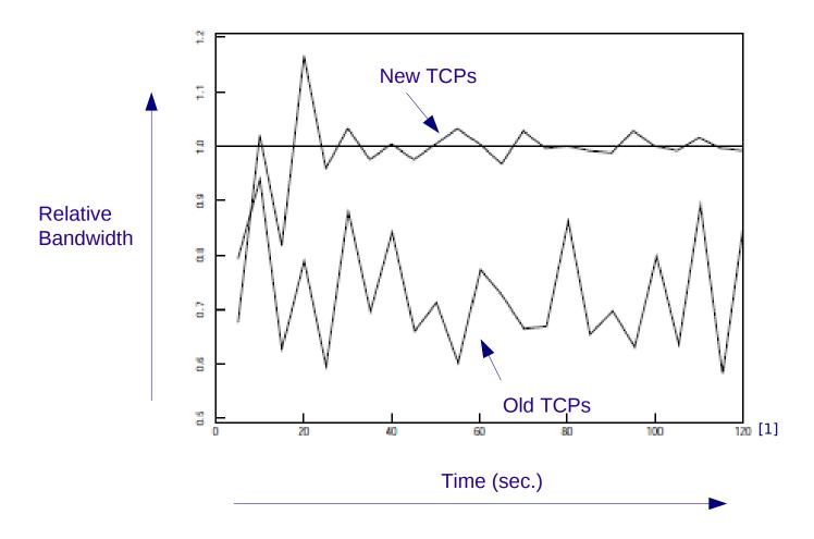
Effective troughput for new TCPs. Window adjustment detail:
