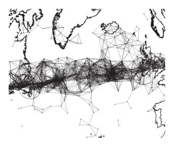
Fig. 9. Example network topology showing how increasing the transmission range reduces the occurrence of local maxima (r = 200 nmi, scenario A).
