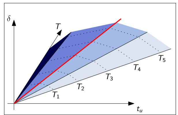
• To find the minimal value of T with  $\delta(T, t_u) \ge 1$  for some  $t_u$ , establish straight line through the highest point of  $\delta(T, t_u)$
