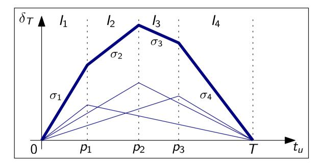
$\sigma_i$  is slope in interval  $I_i$ .
