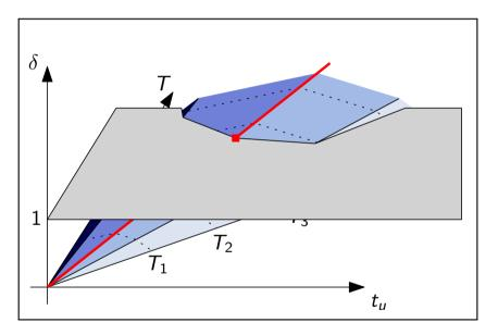
• The decomposition of T into  $t_u$  and  $t_d$  is given by the coordinates of the intersection point.
