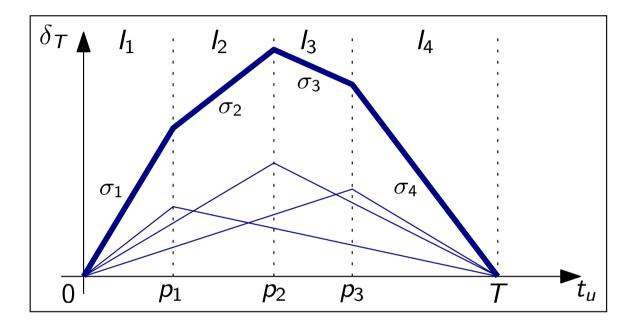
$\sigma_i$  is slope in interval  $I_i$ .
