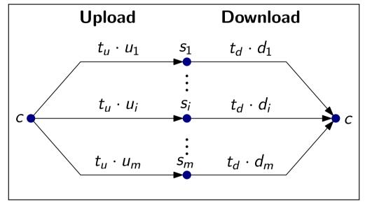
• The maximal amount of data that can be uploaded within  $t_u$  and downloaded within  $t_d$  corresponds to a maximum flow.
