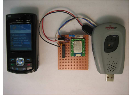
(f) BikeNet mobile SAP implementation. The Nokia N80 Bluetooth radio associates with a custom-built Bluetooth/802.15.4 gateway.
