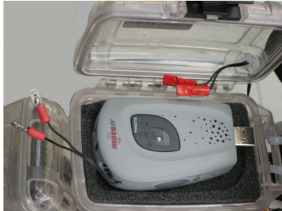
(d) Waterproof OtterBox. Wires are fed through drilled holes that are then filled with silicone sealant. Wires have crimped connectors for easy disconnect.
