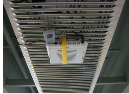
(c) A BikeNet static SAP is a WiFi AP with an Invent inserted in the USB port.
