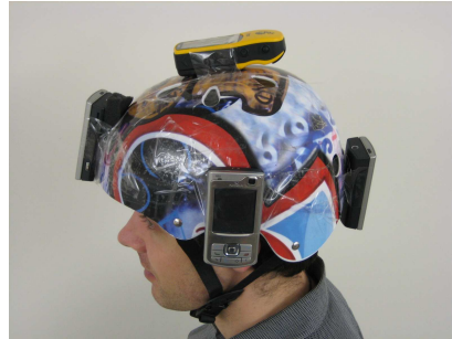
(e) Ground truth video/sound/photo helmet with four N80s and GPS receiver, only for use in debugging our system and validating our inference techniques.
