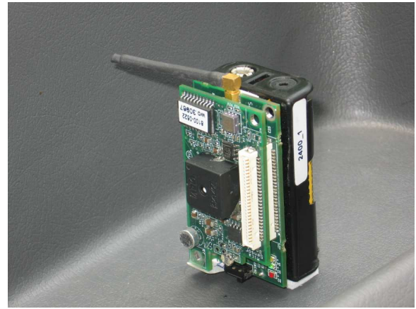
Figure 3: A MICAz mote with a sensor board mounted inside a car.
