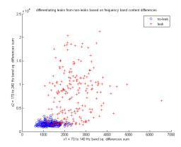
Figure 8: Differentiating Leaks based on differences in frequency band content (sensor 2)
