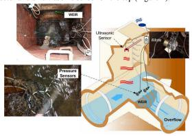
Figure 2: Monitoring the water level in CSOs
