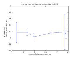
Figure 9: Localization error versus sensor separation
