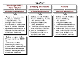
Figure 5: Monitoring system for water transmission pipelines
