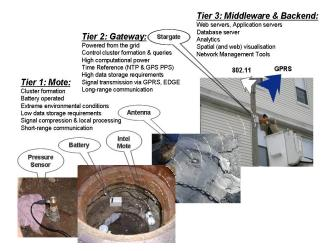
Figure 1: Overview of PipeNet Deployment
