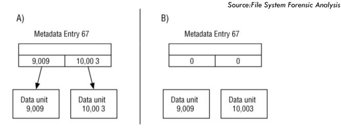
(A) the block pointers are not wiped when the entry is unallocated and in (B) they are wiped
