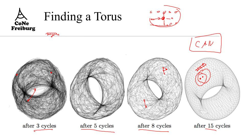
Fig. 2. Illustrative example of constructing a torus over  $50 \times 50 = 2500$  nodes, starting from a uniform random topology with c = 20. For clarity, only the nearest 4 neighbors (out of 20) of each node are displayed.
