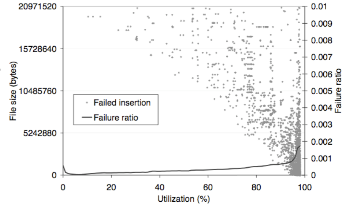
Figure 7: File insertion failures versus storage utilization for the filesystem workload, when t_{pri} = 0.1 , t_{div} = 0.05 .
